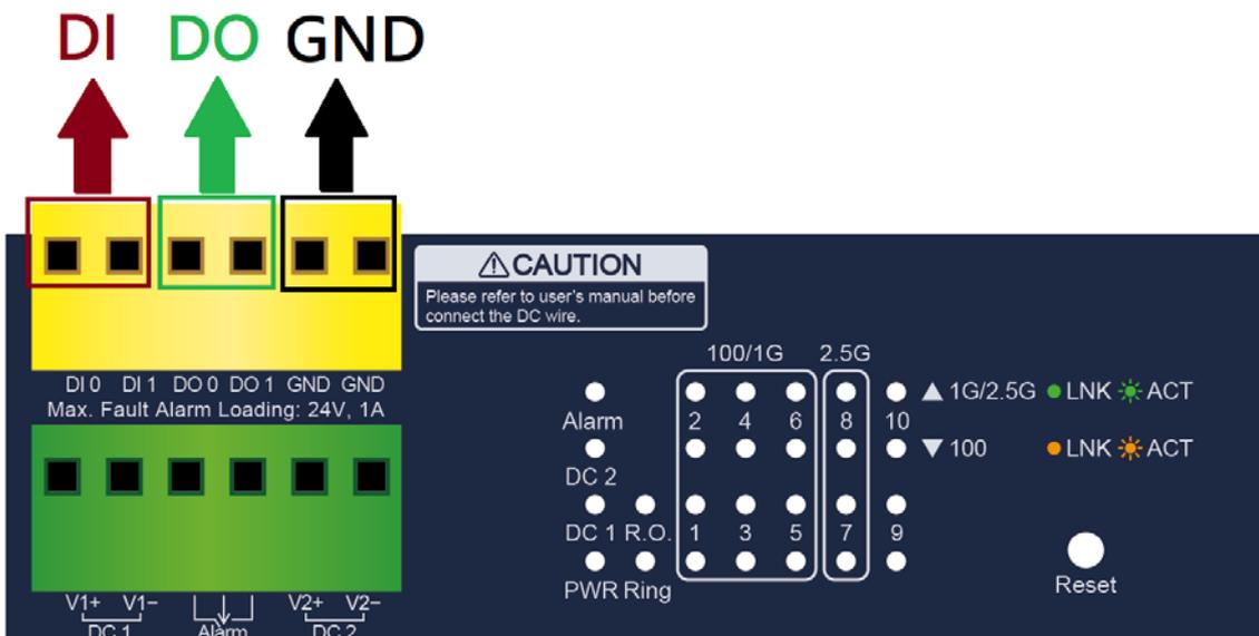
Figure 2-3: Wiring the Digital Input/Digital Output and Ground
