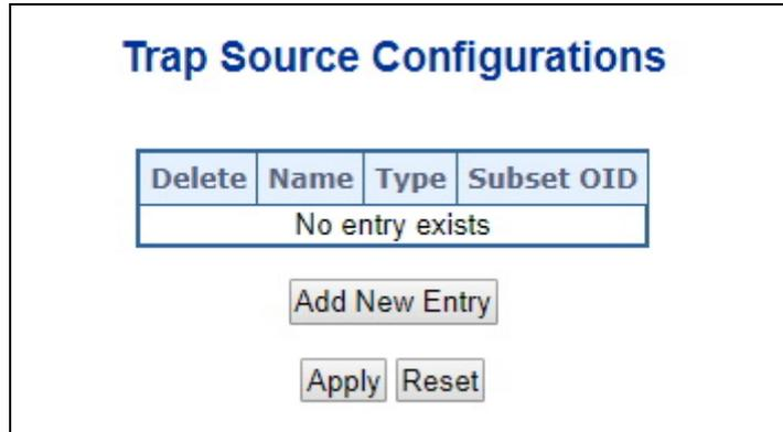
Figure 4-2-2-5: SNMP Trap Source Configuration Page Screenshot
