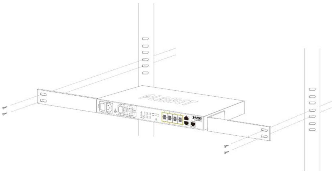
Figure 2-9: Mounting the Managed Metro Switch on a Rack
