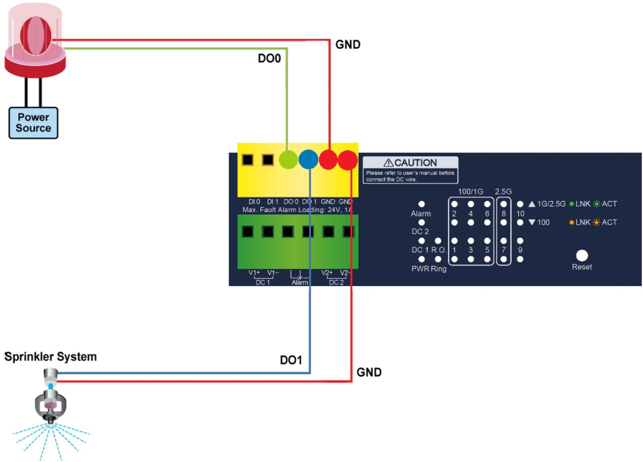
Figure 2-6: Wiring DO0 and DO1 to Open Detector
