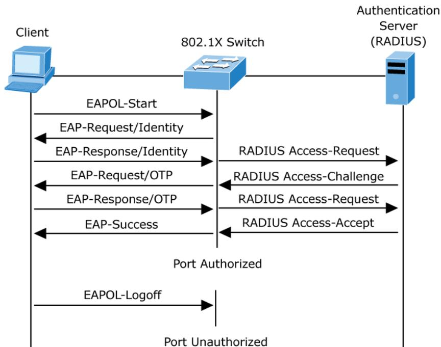
Figure 4-5-2-2: EAP Message Exchange
