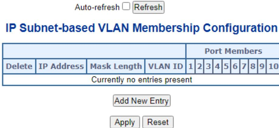
**Figure 4-3-3-17:** IP Subnet-based VLAN Membership Configuration page screenshot
