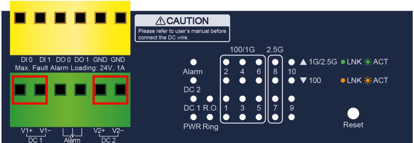
2. Tighten the wire-clamp screws for preventing the wires from loosening.
