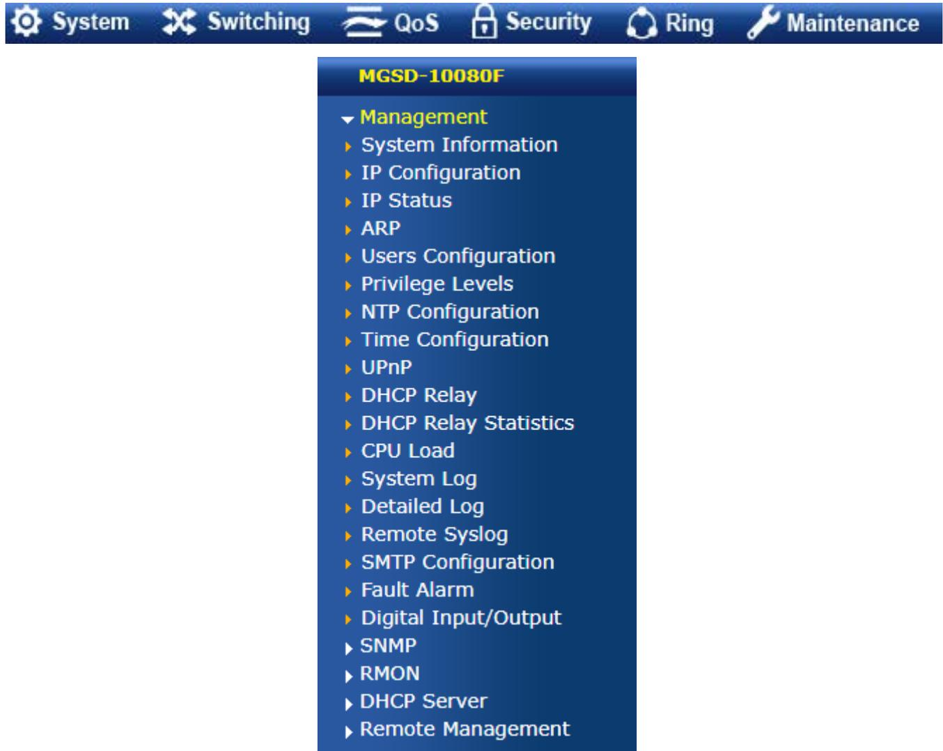
Figure 4-1-5: Managed Metro Switch Main Functions Menu
