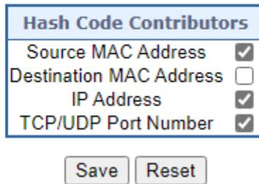
**Figure 4-3-2-2** : Aggregation Mode Configuration Page Screenshot
