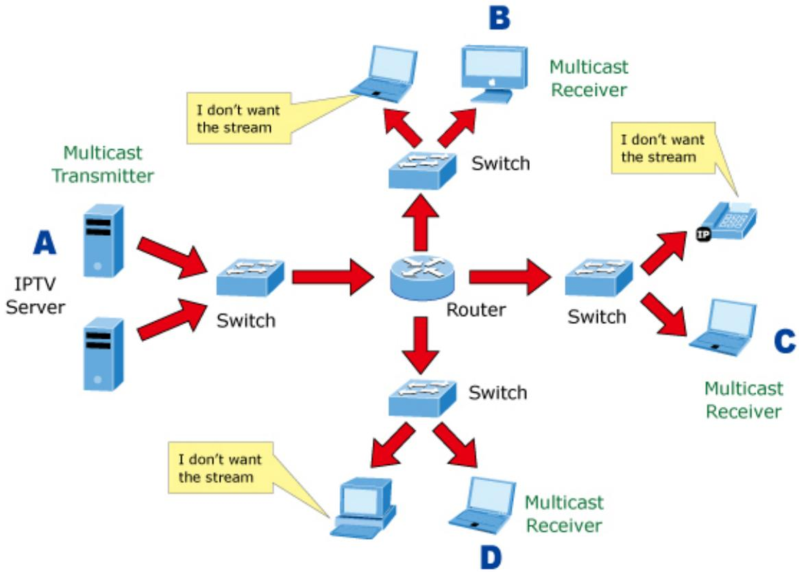
Figure 4-3-5-2: Multicast Flooding
