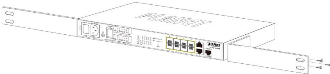
Figure 2-8: Attach Brackets to the Managed Metro Switch.
