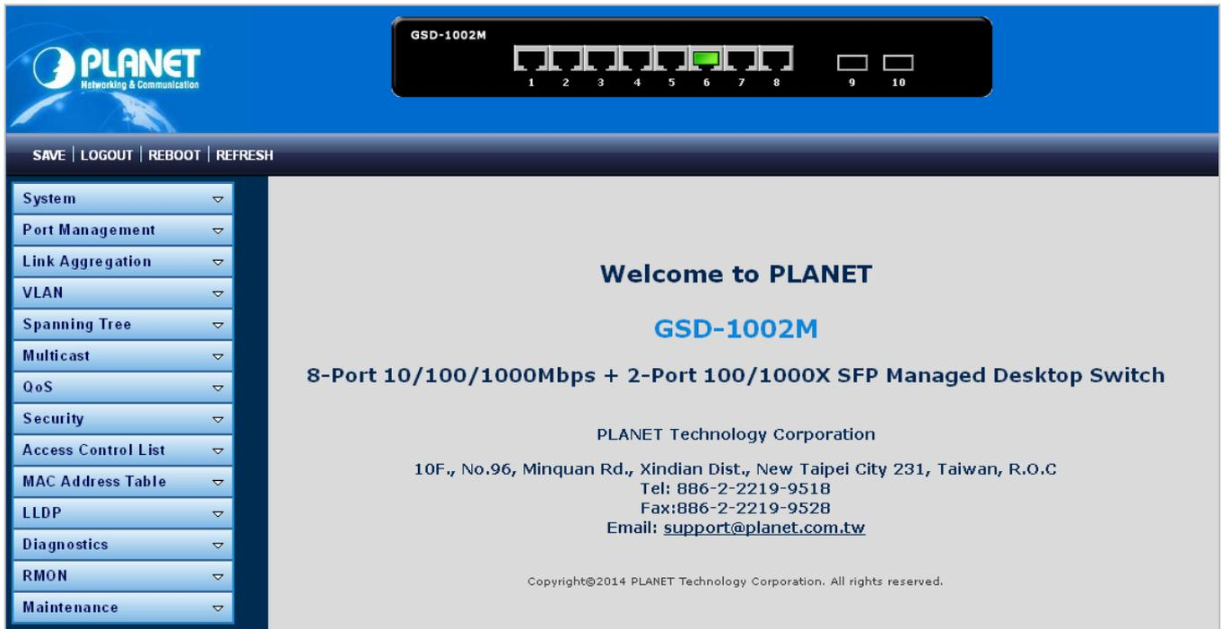
Figure 3-2 Web main screen of Managed Switch
