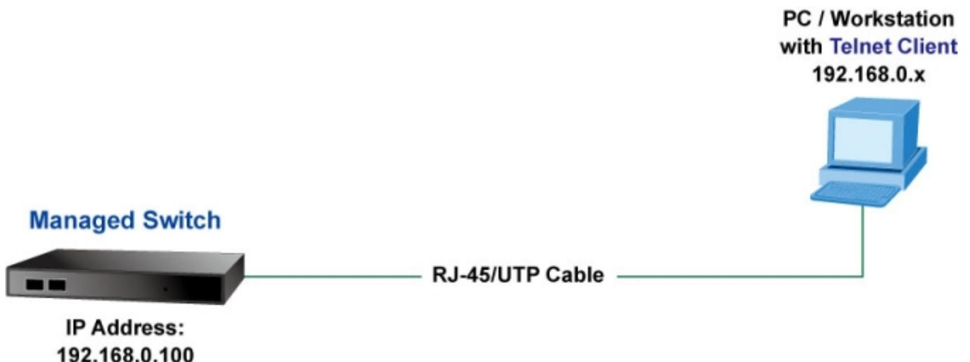
Figure 3-2: Remote Telnet Interface Management
