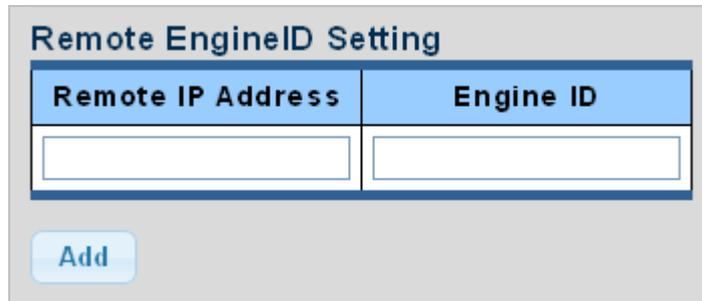
Figure 4-2-37 SNMPv3 Remote Engine ID Setting page screenshot
