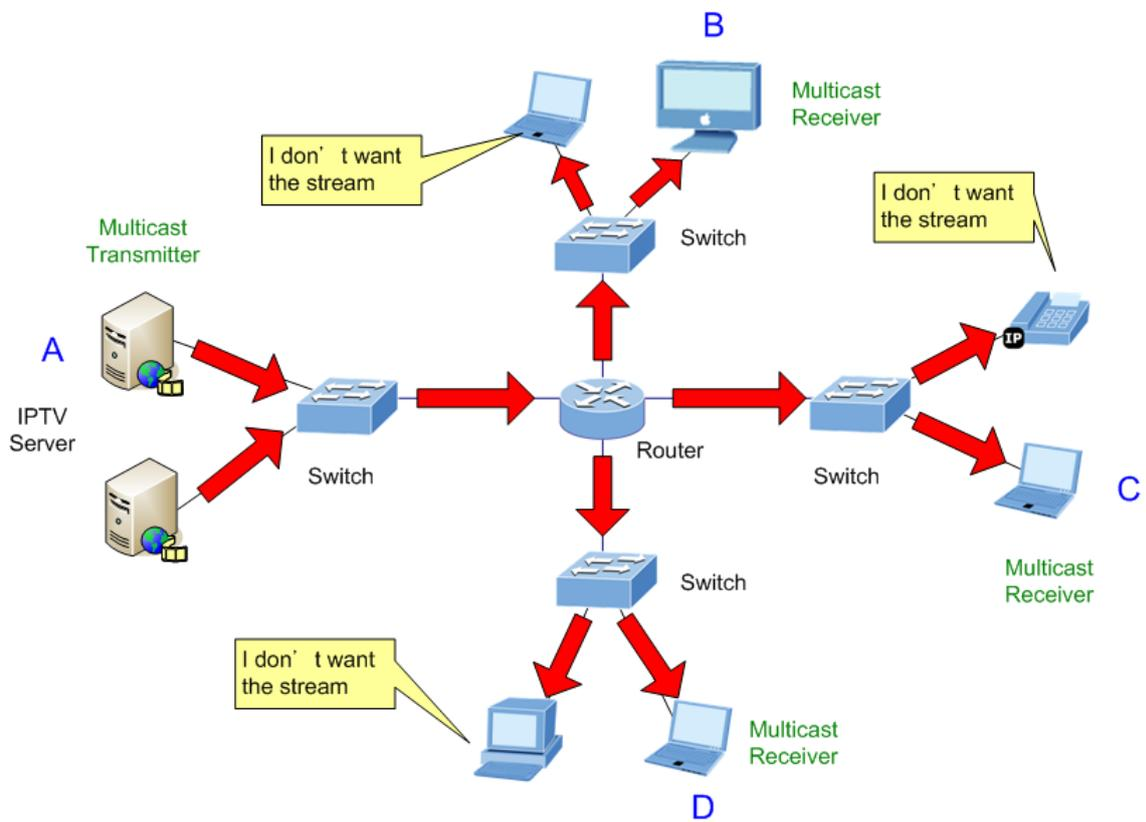
Figure 4-7-4 Multicast flooding
