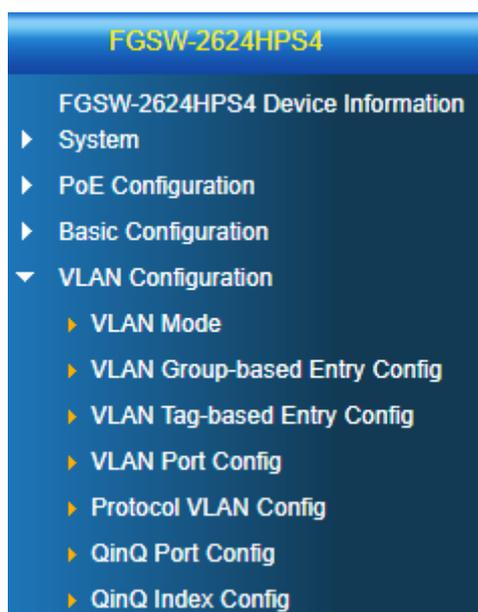
**Figure 4-5-1:** Managed PoE+ Switch VLAN Configuration Web Page
