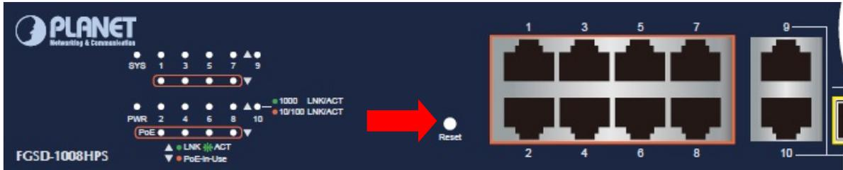
Figure 9-1: FGSW-1008HPS Reset Button
